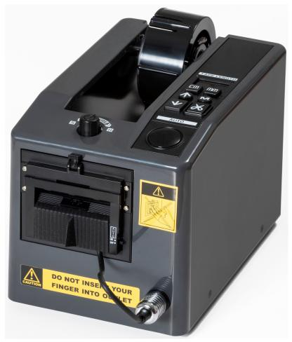
Self-adhesive tapes based on fabric or film with a width of 8-50 mm can be cut with millimeter precision using this device. The tape length is infinitely programmable from 20 - 999 mm.
