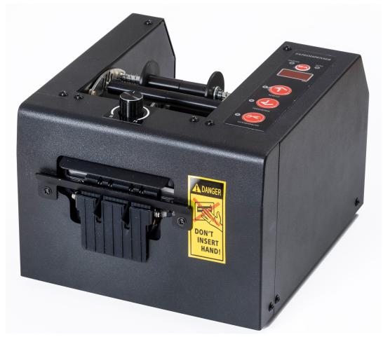
Self-adhesive tapes based on fabric or film with a width of 8-80 mm can be cut with millimeter precision using this device. The tape length is infinitely programmable from 20 - 999 mm.
